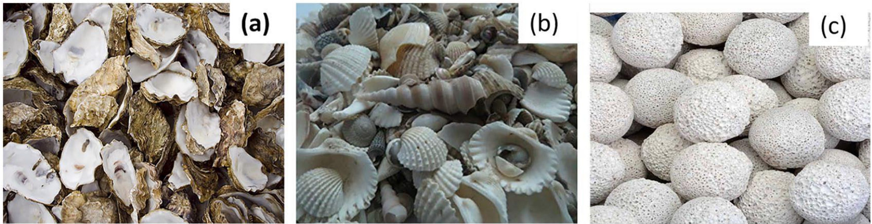
Typical biofilter media from waste shells for wastewater treatment: (a) oyster shells; (b) mixed waste shells biomaterials; and (c) shaped waste shell powder
